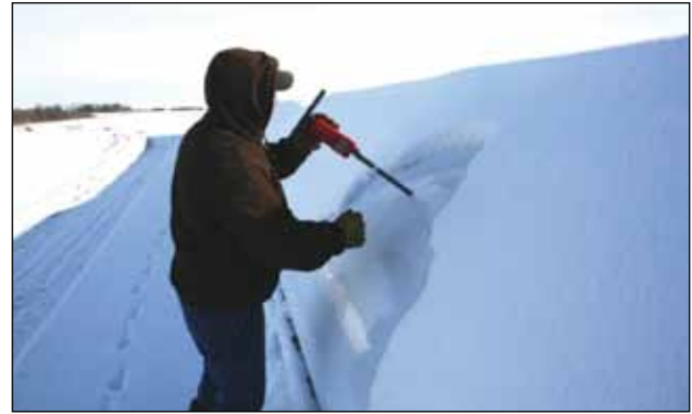
Use of temperature probe (Photo source: Tom Boyle)
