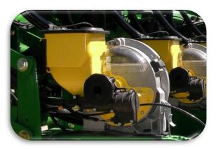
4. If a ½-mile plot length is required, add a hopper extension (D - below). It is OK to stack up to two hopper extensions.
