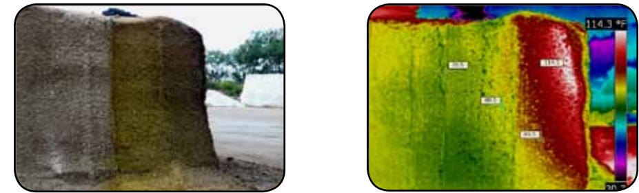
Figure 2. Normal and thermal-sensitive images of a well-managed, split-corn silage bunker showing heat produced from air penetration.
